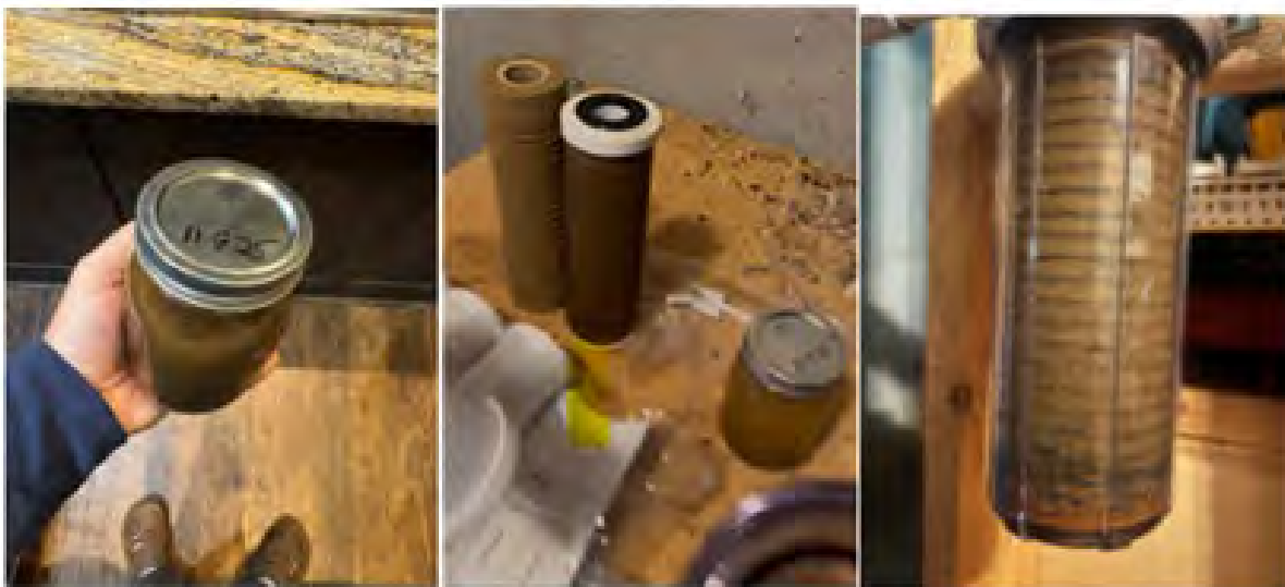
Nov. 9, 2025 (sediment-clogged filters)
